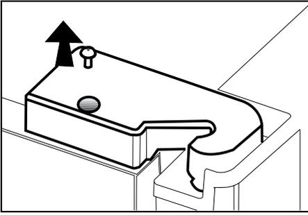
**i** Using a screwdriver, remove the screw of upper hinge cover of the door you want to adjust.
