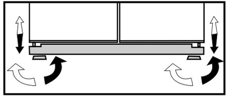
2. After the balance issue is remedied, install back the ventilation cover and fasten the screws.
