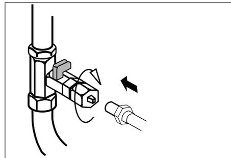
**⚠ Caution:** After turning on the water valve, make sure that there is no leakage at both connection points of the water pipe. In case of a leak, turn off the valve immediately and tighten all joints again using a spanner or a pair of pliers.
