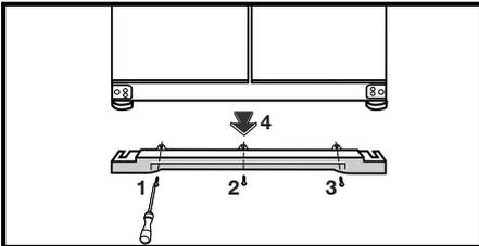
1- Ventilation cover is removed by unscrewing its screws as illustrated in the figure before the procedure.
