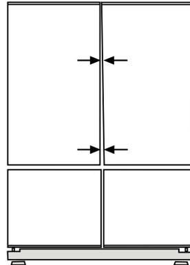
**i** You can adjust the gap between the fridge compartment doors as illustrated in the figures.
