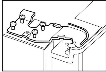
**i** Fix the door you have adjusted by tightening the screws without changing the position of the door.
