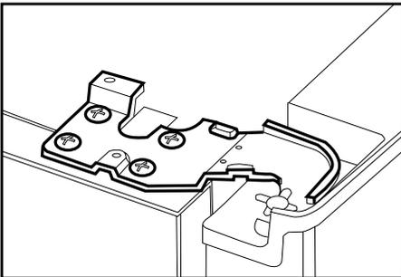
**i** Adjust the door appropriately as you desire by loosening the screws.
