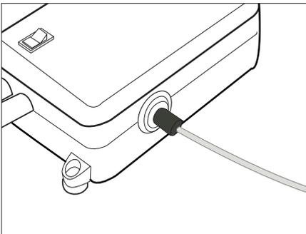
1. Finish the connection by pushing the other end of the water pipe into the water pipe inlet of the pump as shown in the figure.
