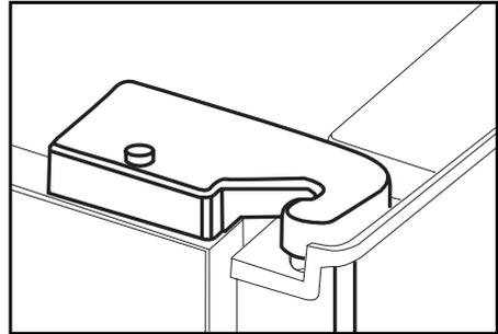
**i** Replace the hinge cover and fix with the screw.
