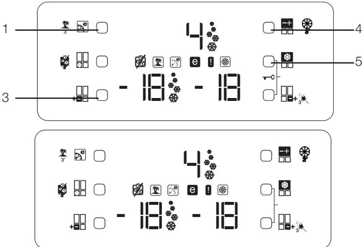
If button configuration is pressed in the correct order, key lock symbol will go off, buzzer will be activated shortly, and Filter change warning indicator illuminates. Press cancel filter change warning button (Item 19 in display descriptions) after changing the filter to have the filter usage time calculated automatically.
